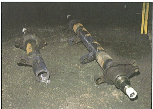
Clean and stripped axles are cut in two.
