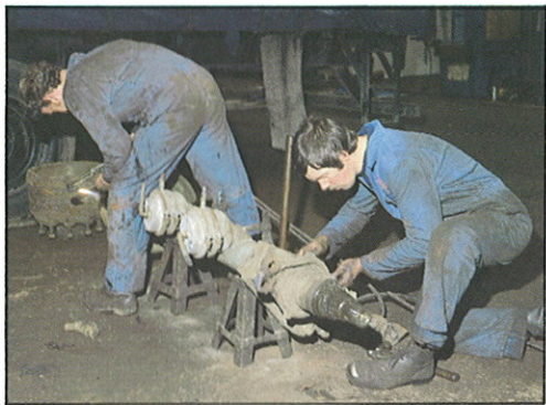
Old axles being stripped for conversion at the Primrose works.
